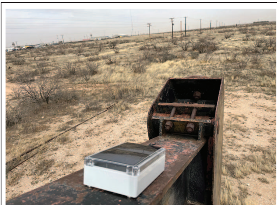
With a solar-powered device that costs less than $2 a day, stripper well operators can count each pumpjack's strokes and determine which ones are no longer running. According to Telemetry Insight, this information helps pumpers prioritize sites that need attention.
